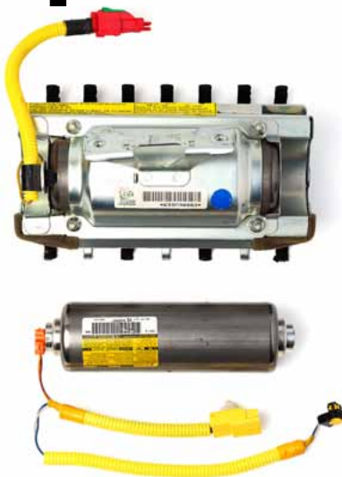
A Takata passenger side airbag assembly and inflator
