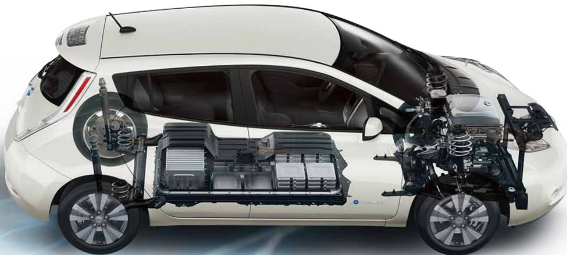
A cross-section of a Nissan Leaf showing its battery
