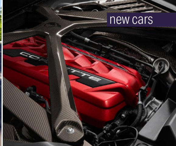
The model-year 2025 Corvette Z06 with the performance package and large rear spoiler. The engine bay housing the 475kW 5.5-litre LT6 features carbon-fibre bracing
