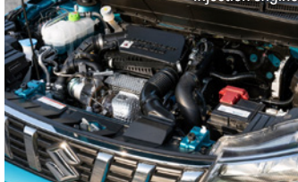
The new K14D version of the 1,372cc Boosterjet direct-injection engine
