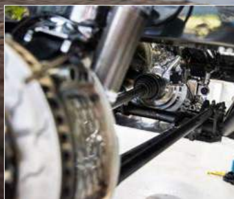
The Hyundai Kona's electric motors are set low in the front and rear of the car. This offers excellent weight distribution and a low centre of gravity
