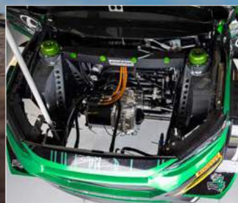
With no internal combustion engine, turbo or intercooler, the front of the car seems empty. Almost all the weight of the motors and batteries is in the wheelbase to further improve handling
