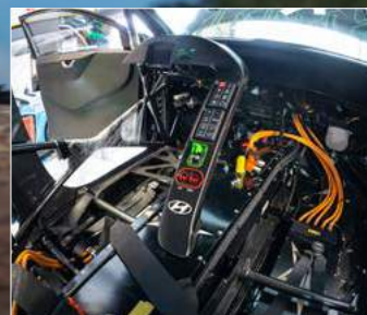
Paddon sits on the left with the custom controller panel easily to hand. To the right and set down on the floor is the EV motors' management array
