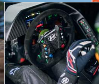
The steering wheel carries controls for functions used most often, while the full-colour Motec display provides Paddon with vital information and data
