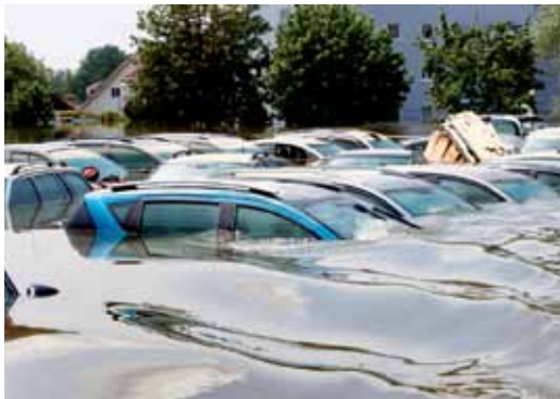
Light vehicles that have been damaged by floods now require all electronic and pyrotechnic safety components to be replaced
