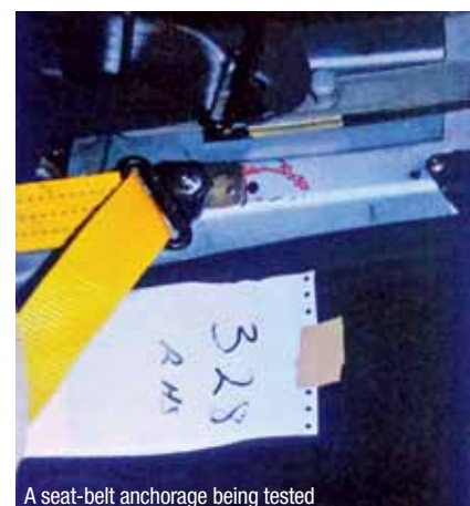
A seat-belt anchorage being tested
